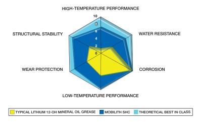
Mobilith SHC shows significantly higher performance compared with a conventional mineral oil-based grease.
