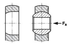
The base in the steel housing is cylindrically turned from one side and, starting from the centre line, it runs to suit the ball's contour (see drawing).
