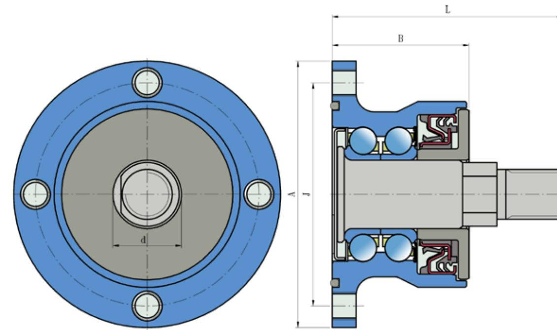
Fig.11. Technical drawing bearing unit IL2-117-M22
