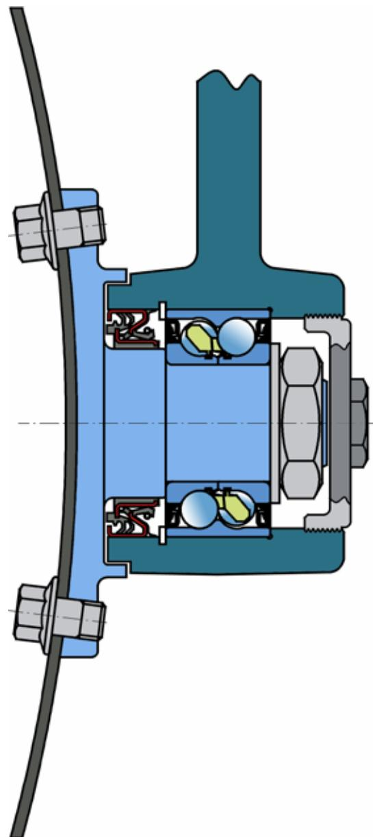
Fig.10. Mounting of disc harrow bearing
